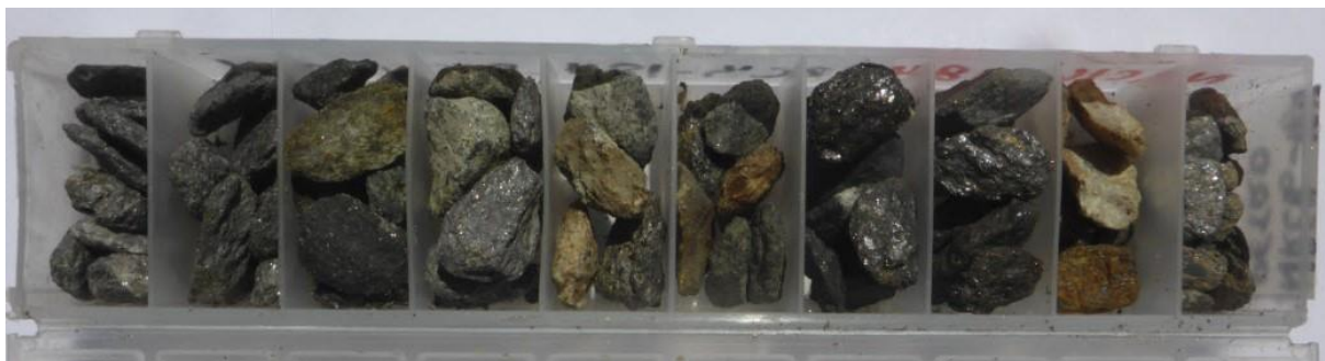
RC drill chips from a graphite deposit. The chips are about 5 mm length. Each compartment in the chip tray represents 1 metre.
